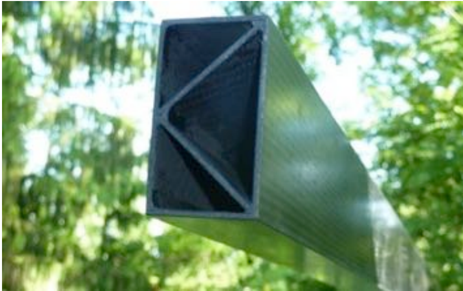
Frame profile for automotive industry from Carbon fibers and African granite
