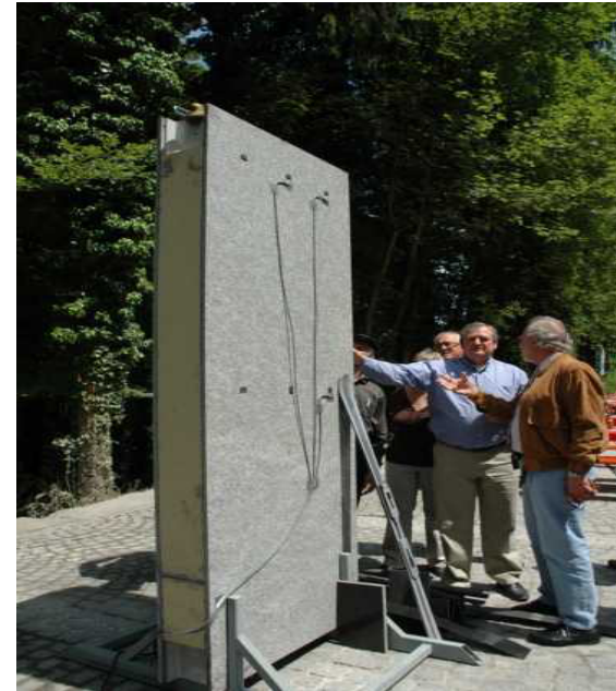
House wall from 20 mm thin MCT® plates with insulation layer from PUR foam between the plates
