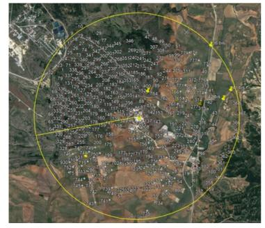
**Above:** Surface view of the ENOS 3D VSP acquired in September 2017 with a grid of 390 surface source points distributed around the injection well at Hontomín, Spain. The yellow circle has a radial distance of 2.1 km from the well (map courtesy OGS, Italy)
